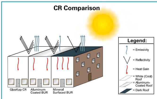
Combining highly reflective and emissive roof surfacing with the proper amount of roof insulation can significantly reduce heat gains inside the building. Keeping the roof cooler also has other advantages, as well. It helps prevent thermal shock: the sudden, drastic change in roof temperature that can cause membrane fatigue.
