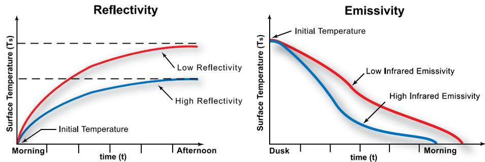
Conceptually, the above graph presents two products – one with high reflectivity, one with low reflectivity. During peak afternoon hours, the product with the higher reflectivity delivers a cooler rooftop surface.
